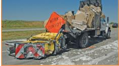
Truck-mounted attenuators before and after a vehicle impact (TTI).
